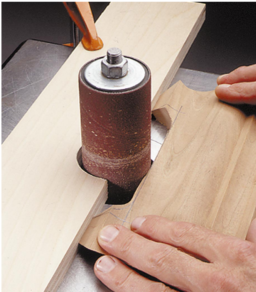
When forming the legs, use a fence with a drum or spindle sander to sand a straight edge and smooth radius.
