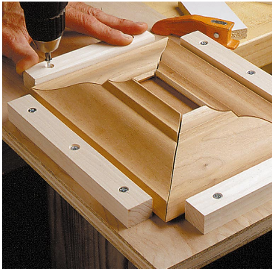
Attach four cleats at right angles to each other to hold the lid pieces in position on a plywood clamping platform.
