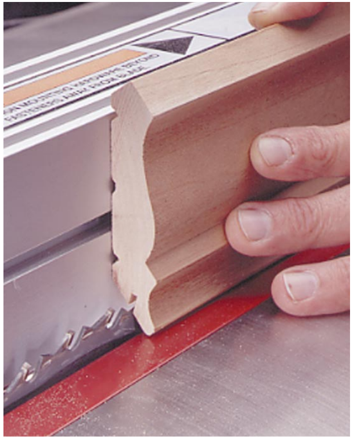
Hold the back side of the molding against your table-saw's fence to cut the kerf that holds the panel in the center of the lid.
